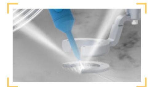
The Water Jet is the cold cutting solution, suitable for shaped pieces with more or less complex geometries up to quite significant thicknesses. A jet of pure water or mixed with abrasive can be used. The cutting unit is assembled on the axis slide (Z) and is composed of a kit of cutting that mixes water and abrasive. The water jet cutting heads used by OMAG guarantee maximum efficiency and minimum maintenance.
